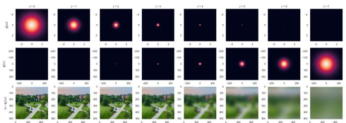
The top row is the Forrica transform of  $\phi_J$ ;  $\hat{\phi}_J(\omega)$ . The middle row is  $\phi_J(u)$ . The bottom row is  $(x + \phi_J)(u)$ . The scales range over  $0 \le J \le 7$ . The low pass function here is a Gaussian;  $\frac{1}{2\pi\sqrt{2}} e^{-\frac{1}{2\pi\sqrt{2}}} e^{-\frac{1}{2}(u)^2/2} \Rightarrow \hat{\phi}(u) = e^{-\frac{1}{2}(u)^2/2}$
